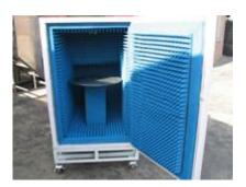
is a wooden box with copperplate or ferrous board in the interspace to shield electromagnetic wave. Absorbers are stuck to the copperplate or ferrous board. Anechoic box is mainly used to test mini-type antenna's or electronic apparatus' capability of receiving &dispatching signals and anti-jamming. Different dimensions of such an anechoic box are available according to customers' requirements.
