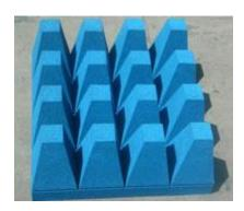
compound absorber material used for EMC anechoic chambers. It consists of thin ferrite tile, matching sheet and conical absorber material. It can provide enough wideband performance to test EMC anechoic chambers at the range of frequency from 30MHz to 30GHz.
