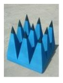
aligned light blue quadrangular pyramid, possessing good fireproof performance which fulfills American NRL Report 8093. Service temperature: -50  $^{\circ}$ C  $\sim$  70  $^{\circ}$ C . It is of good vertical incidence  $^{\circ}$  oblique incidence  $^{\circ}$  scattering and isolated decay performances at the wideband range. It is mainly used for subject material of anechoic chambers.
